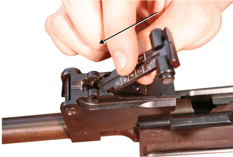
Figure 47. Installing the Rear Sight Assembly.
