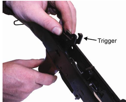
Figure 37. Installing the Trigger.
