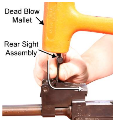
Figure 10. Dislodging and Removing the Rear Sight Assembly Using a Dead Blow Mallet.
