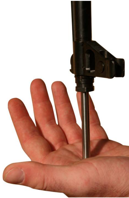
Figure 10. Bore Straightness Gage Coming out of the Muzzle.
