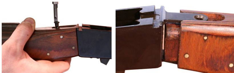
Figure 28. Removing Buttstock Screws and Pulling the Fixed Buttstock from the Receiver.
