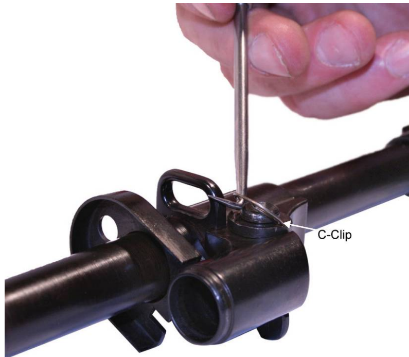
Figure 6. Removing the C-Clip with the Scraper Tool.
