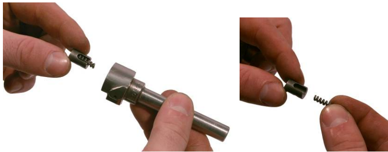
Figure 4. Removing the Extractor and Extractor Spring.
