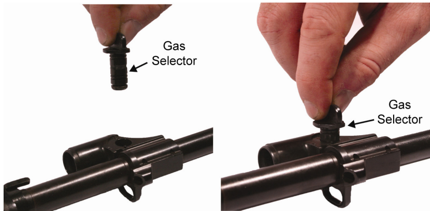
Figure 48. Installing the Gas Selector.
