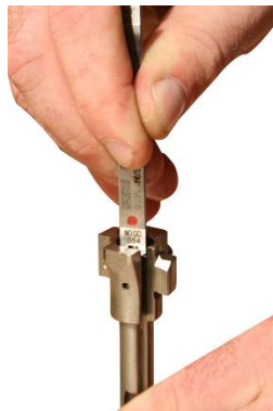
Figure 4. Using the “No-Go” Side of the Firing Pin Protrusion Gage.
