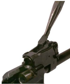
Figure 46. Installing the Rear Sight Leaf Spring.
