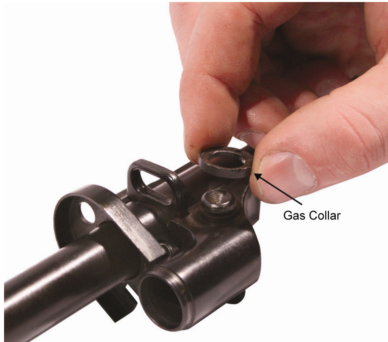
Figure 49. Installing the Gas Collar.
