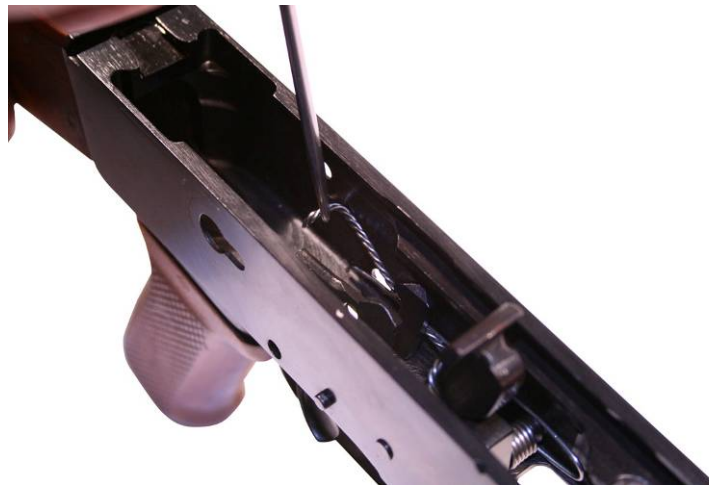
Figure 38. Lowering the Hammer Spring Legs onto the Trigger.
