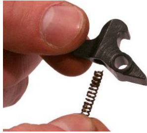
Figure 18. Removing the Disconnecter Spring from the Disconnecter.
