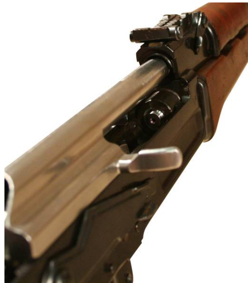
Figure 17. Headspace “No-Go” Gage Fully Seated in the Chamber.
