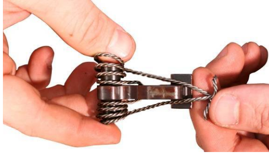
Figure 23. The Hammer and Hammer Spring Removed.
