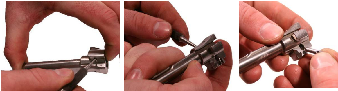
Figure 3. Removing the Grooved Extractor Retaining Pin.
