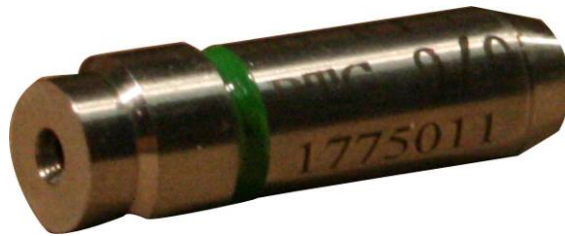
Figure 11. The Headspace “Go” Gage.
