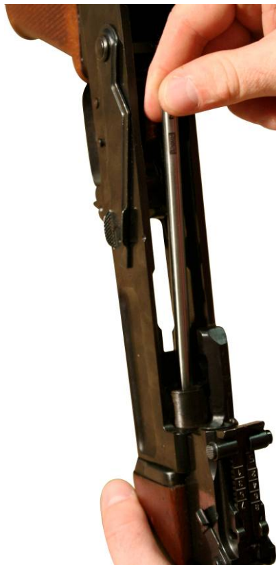
Figure 9. Dropping the Bore Straightness Gage through the Chamber.
