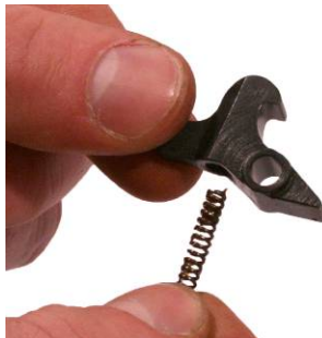
Figure 40. Installing the Disconnecter Spring.
