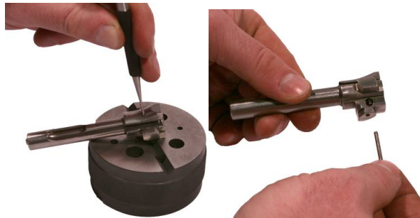
Figure 1. Removing the Firing Pin Retaining Pin.
