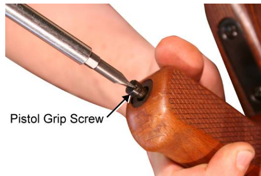
Figure 27. Removing the Pistol Grip Screw.
