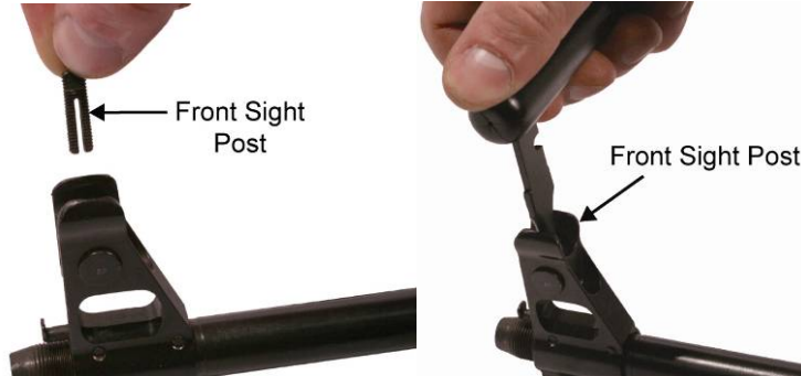
Figure 53. Installing the Front Sight Post.
