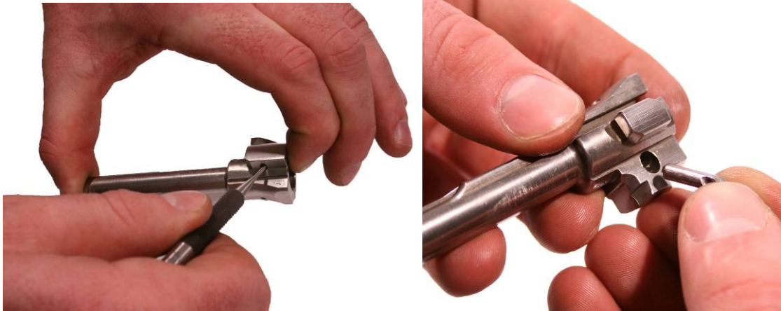
Figure 7. Installing the Grooved Extractor Retaining Pin.
