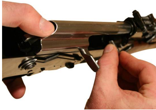
Figure 12. Inserting the Headspace “Go” Gage.
