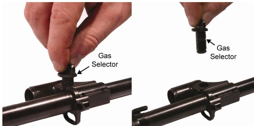
Figure 8. Removing the Gas Selector.
