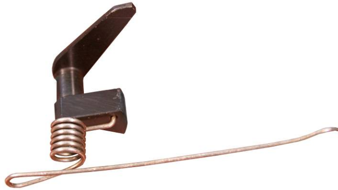
Figure 33. The Short Leg of the Auto Sear Spring Installed in the Auto Sear.
