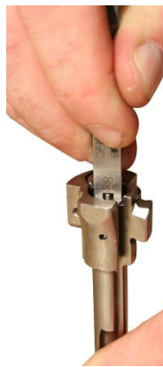
Figure 3. Using the “Go” Side of the Firing Pin Protrusion Gage.
