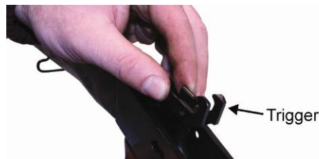
Figure 36. Trigger with Dual Hammer Hooks.
