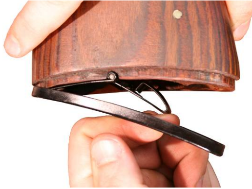
Figure 2. Removing the Buttplate and Trap Door.
