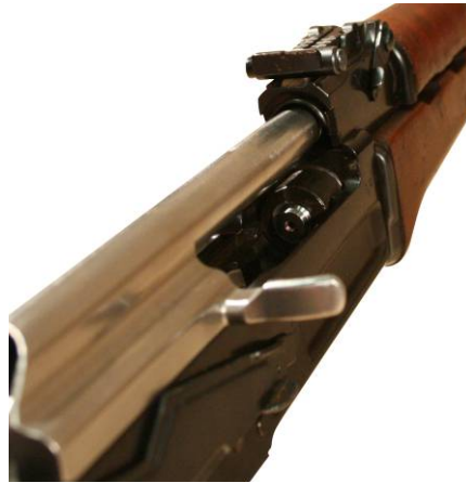
Figure 13. Headspace “Go” Gage Fully Seated in the Chamber.
