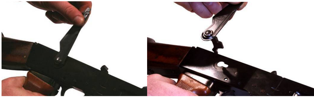
Figure 19. Rotating and Removing the Selector Lever.
