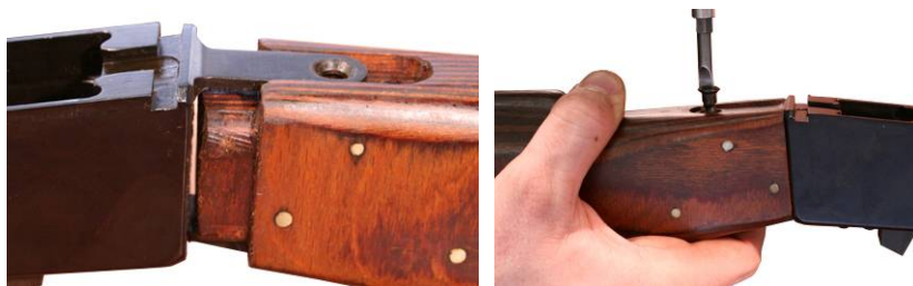
Figure 30. Aligning and Installing the Fixed Buttstock onto the Rear of the Receiver.
