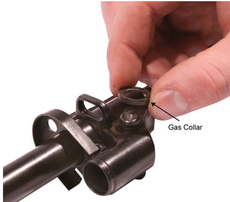
Figure 7. Removing the Gas Collar.
