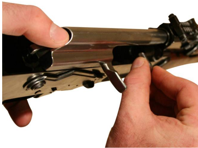
Figure 16. Inserting the Headspace “No-Go” Gage.
