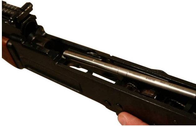
Figure 6. Inserting the Bore Erosion Gage into the Breech End of the Barrel.
