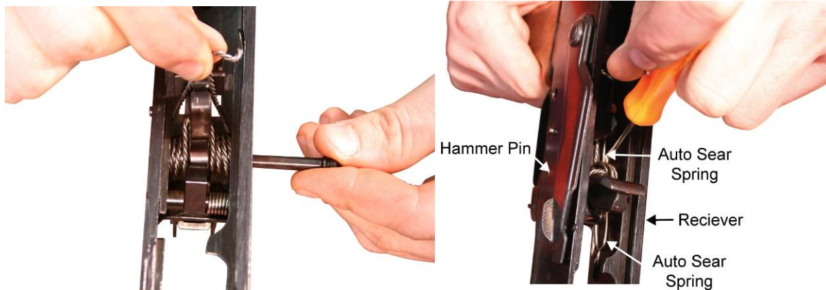
Figure 35. Installing the Hammer Assembly and the Hammer Retaining Pin and Setting the Auto Sear Spring into Groove of the Hammer Retaining Pin.
