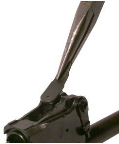
Figure 12. Removing the Rear Sight Leaf Spring.
