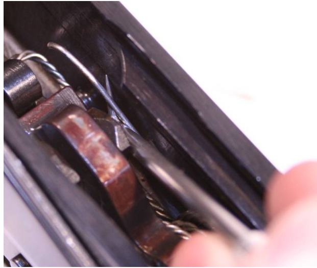
Figure 14. Removing the Long Leg of the Auto Sear Spring from the Groove in the Trigger Retaining Pin.
