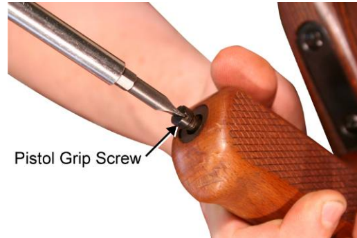
Figure 31. Installing the Pistol Grip.
