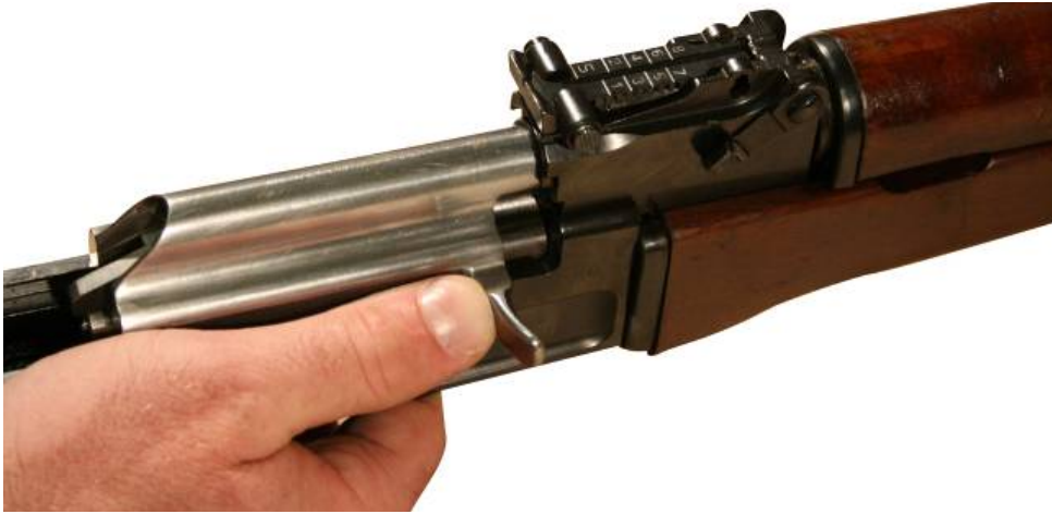
Figure 18. Bolt NOT Locked.
