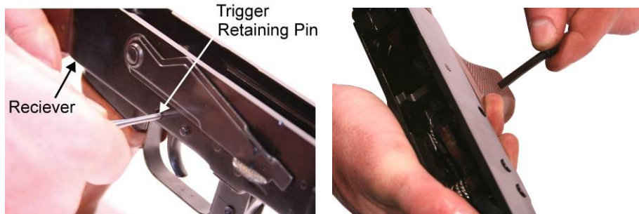
Figure 16. Using a Punch to Push Out the Trigger Retaining Pin.
